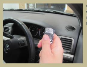
Our remote control systems all have a "Rolling Code System" which means it's virtually impossible to copy the frequencies of your handset thus enabling access to your garage.
